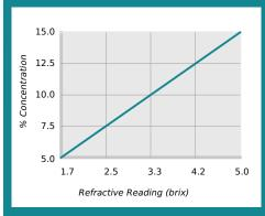
% Concentration = Refractive Reading x Refractive Factor Coolant Refractometer Factor % Brix = 3.0
