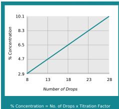
% Concentration = No. of Drops x Titration Factor Titration Factor = 0.36
